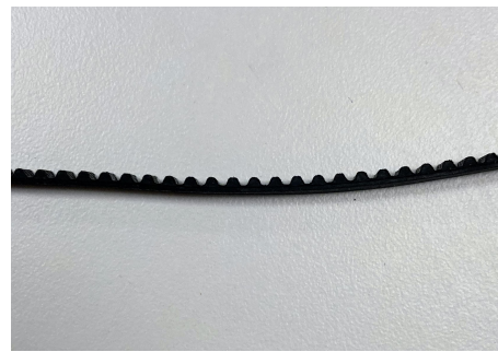
Figure 3.7: Chloroprene rubber with fiberglass reinforcements toothed belt.
