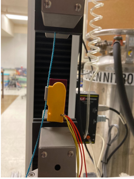
Figure 4.1: Ratchet latch clamped into tensile testing machine.
